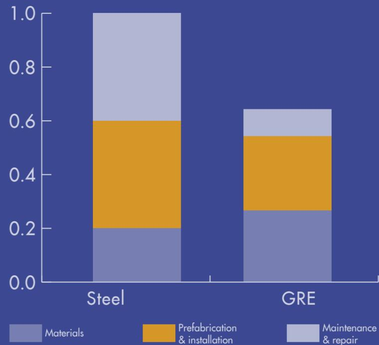
Although the GRE material cost is higher than steel material, the total installed cost of GRE is similar to steel piping. Moreover, mounting GRE will contribute to lower through life cost.
